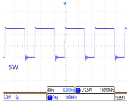
Fig 4 SW Waveform
