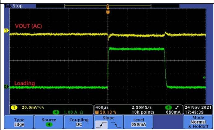
Fig 4. Load Transient, I<sub>OUT</sub>=0A to 3A
