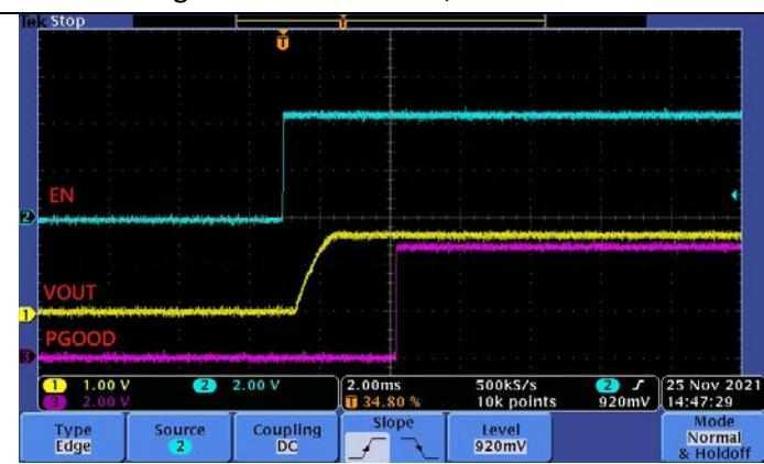
Fig 3. EN Power ON, I<sub>OUT</sub>=200mA
