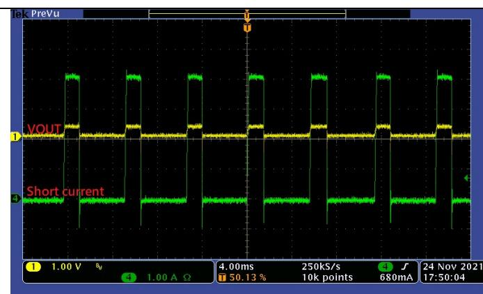
Fig 5. VOUT Short circuit
