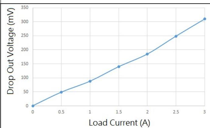
Fig 6. VDROP vs Output Current
