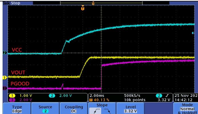
Fig 1. VCC Power ON, I<sub>OUT</sub>=200mA
