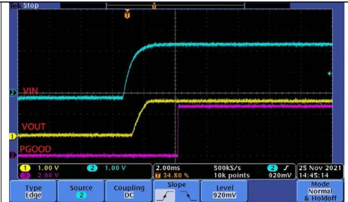
Fig 2. VIN Power ON, I<sub>OUT</sub>=200mA
