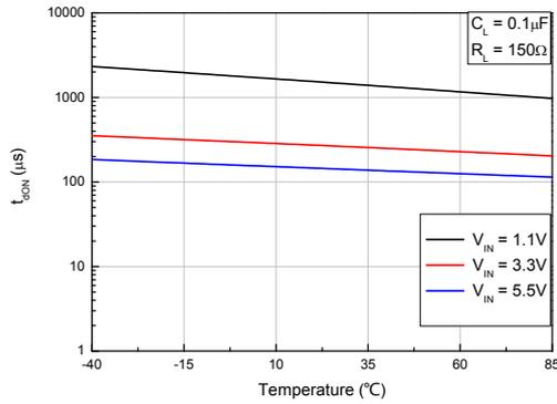
Fig. 11  $t_{dON}$  vs. Temperature (HM9708A)
