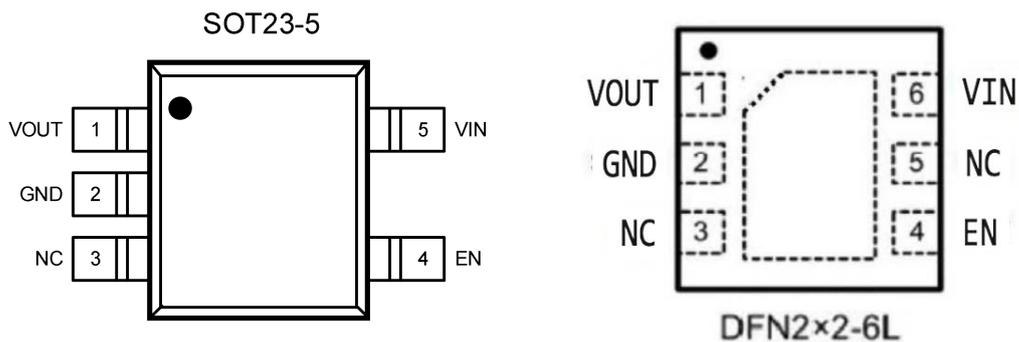
Fig. 2 Pin configuration
