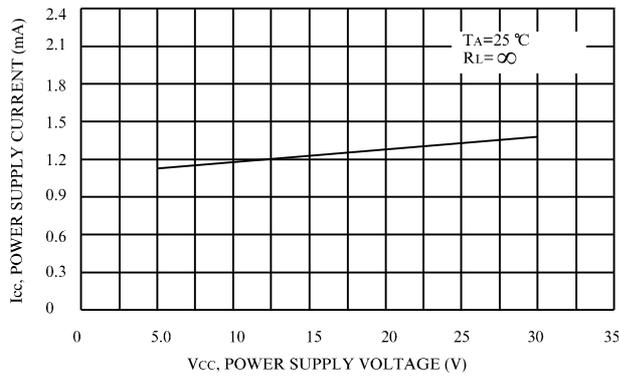
Figure 5. Power Supply Current versus Power Supply Voltage
